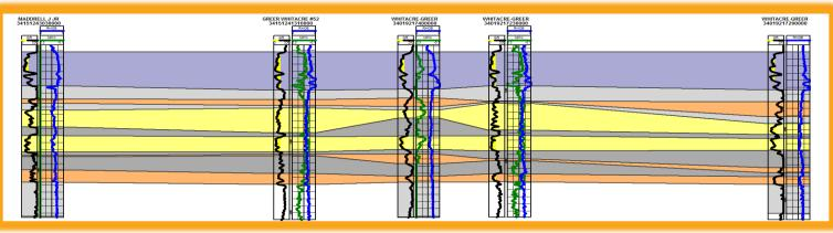
A cross section through multiple wells of ECOF zones and layers. Yellow/orange zones represent sands and gray zones represent maximum flood surfaces.
