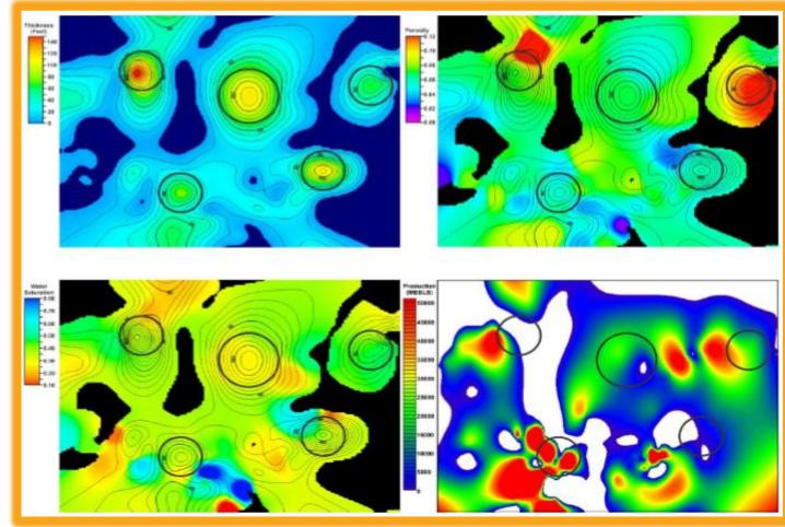
Isopach (A), average porosity (B), average water saturation (C), and cumulative production (D) maps for Copper Ridge Dolomite Reservoir using the moving average method.
